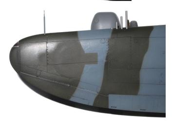
Replacement decals were done like the originals - Future for gloss coat underneath, apply decals with Micro-Set, clean residue, seal with Future, sand edges, and seal again. Finally the areas were restored with a final coat of Testors Dullcoat.
